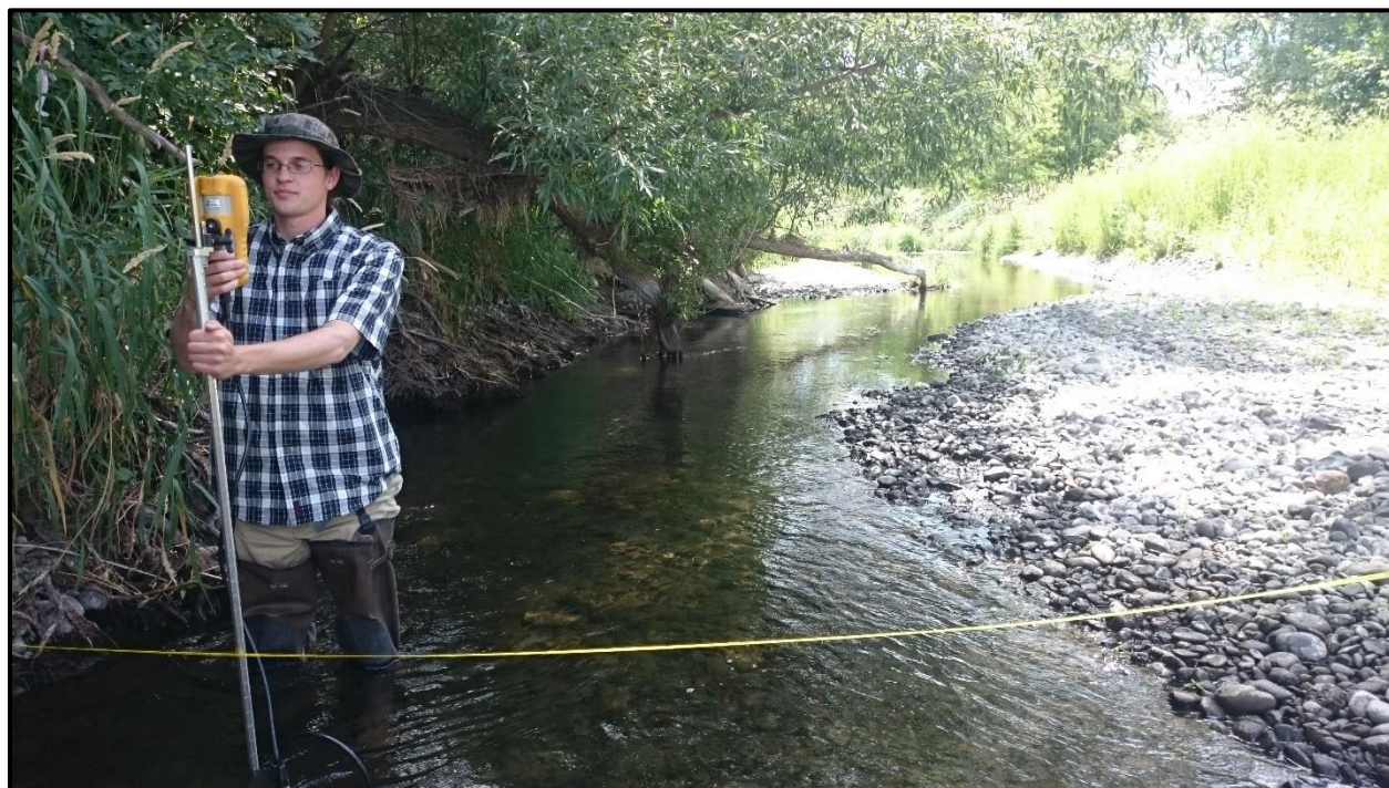
Figure 5. Staff taking a wading flow measurement on Mill Creek using a FlowTracker2.
