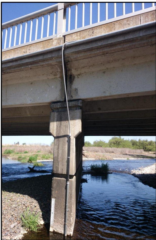
Figure 4. At this near real-time monitoring site on Mill Creek, flexible conduit secured to a bridge pier protects a sensor and cable that collect and transmit water level data to a communications box equipped with a solar panel, battery and an antenna, which utilizes radio telemetry to transmit data to the WWBWC office to be processed and published online.
